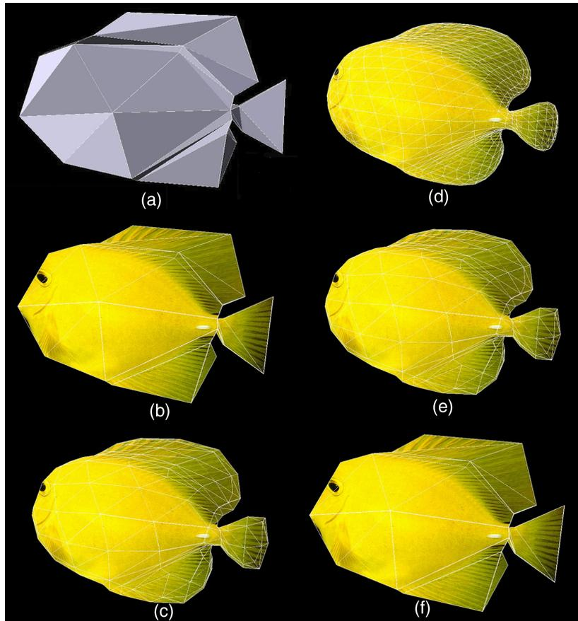
Figure 14: (a) *The control mesh.* (b) *The textured control mesh.* (c) *The resulting mesh after one step of Loop subdivision.* (d) *After two steps of Loop subdivision.* (e) *The resulting mesh after applying the reverse scheme on mesh (d).* (f) *The resulting mesh after applying the reverse scheme on mesh (e).*
