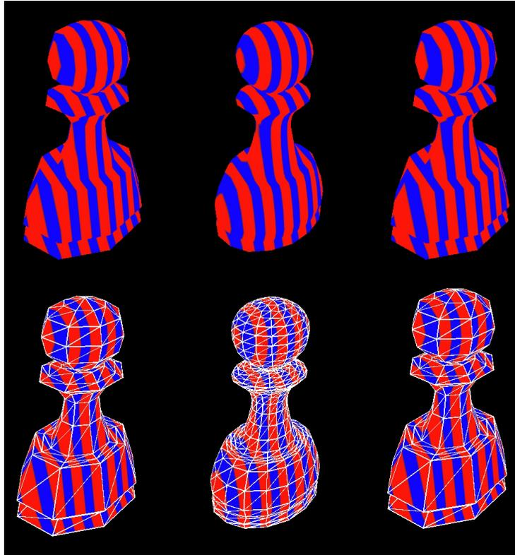
Figure 10: *The top-left shows the textured control mesh of a pawn, and the top-middle is the fine mesh obtained by Loop subdivision, and top-right shows the obtained mesh from the reverse process. The second row shows the same meshes together with grid lines.*
