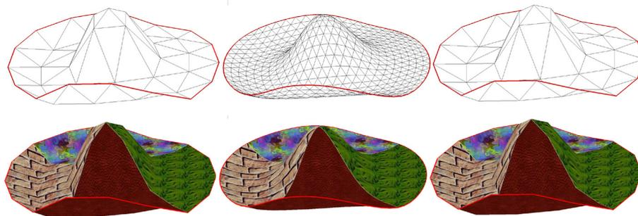
Figure 11: *The top-left shows a simple control mesh with boundary, and the top-middle is the fine mesh obtained by Loop subdivision, and top-right shows the obtained mesh from the reverse process. The second row shows the same meshes together with a simple texture.*
