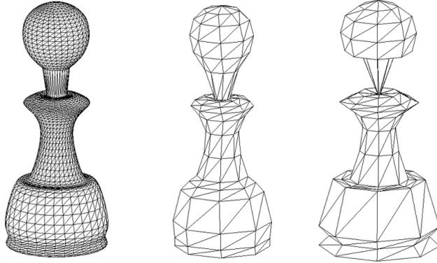
Figure 13: *The left shows a modified fine mesh of the pawn, and the middle is the resulting coarse mesh via the mask 10, and the right shows the obtained mesh from the reverse Loop.*
