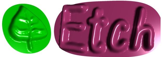
Figure 4. Creating a leaf and writing some letters onto a subdivision surface. The constraints for the veins of the leaf and the letters were generated using an etch tool, which placed constraints on the surface to match a user’s mouse movement.
