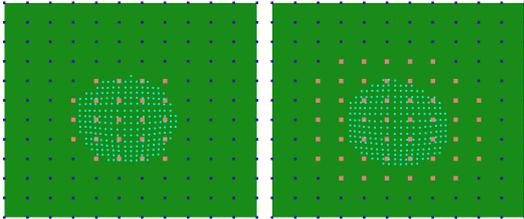
Figure 1. The same set of blue constraints are given, and the selected set  $S$  is shown in red. Left: Choosing only the maximal basis functions. Right: Choosing all non-zero basis functions.
